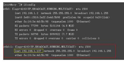
The command output in the preceding figure contains a network interface named **eth***X*:*X*. **192.168.1.137** is its virtual IP address.
