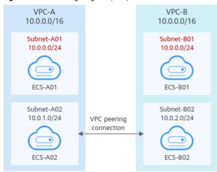
Figure 4-5 Networking diagram (IPv4)
