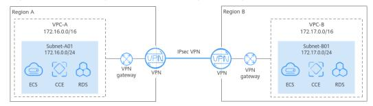
Figure 7-1 Connecting VPCs in different regions using VPN
