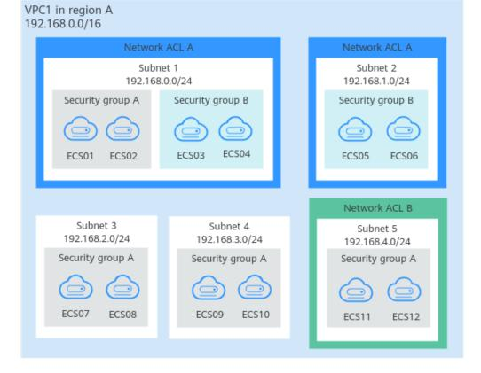
Figure 2-2 Communications between subnets in a VPC
